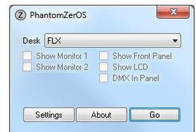
Now ensure “Show Front Panel” and “Show Monitor 1” is ticked on the window shown to the right. On the front panel, click the “SETUP” button. On the LCD, choose “Load File” and select the .isf file you saved onto the desktop earlier.
